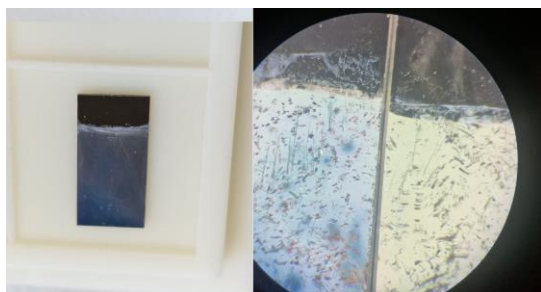
Fig. 1: On the left, photograph of 10 N ZIF-8 thin film on silicon substrate. On the right, 5 N and 10 N ZIF-8 thin films on silicon substrates under microscope.
