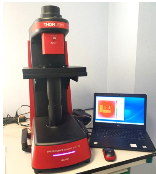
Fig. 3. Birefringence imaging system (BIS).
