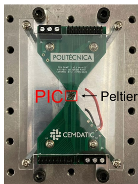
Fig. 6: Proposed PIC packaging for the device testing. PIC: Photonic Integrated Circuit.
